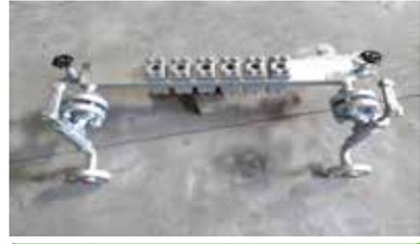
**Steam Drum level gauges & its spares.**
