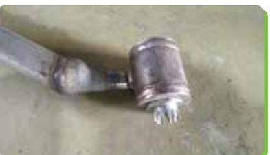
**Spent Wash Fired Boiler-Spent Wash Gun Assembly With Flexible Hose**
