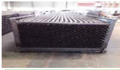
**ESP Collecting & Discharge Electrode.**
