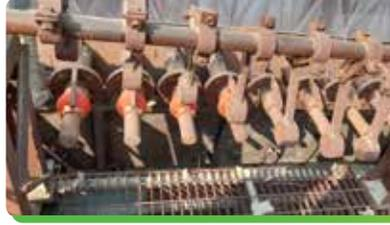
**Spent Wash Fired & Cement WHR Boiler Rapping Hammering System & It's Spares**
