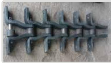
**Travagrate Boiler Chain & its Internal Spares :**
