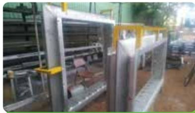
**Boilers Ducting Metallic Expansion Joints- Single Loop/Double Loop**
