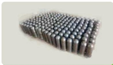
**AFBC & Spent Wash fired Boiler Air Nozzles & Bubble Caps**
